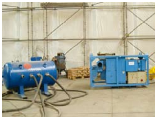
(1) A new bridge is being painted in the workshop before transportation. An enclosure protects the fresh paint from the environment and a dehumidifier regulates the climate.
