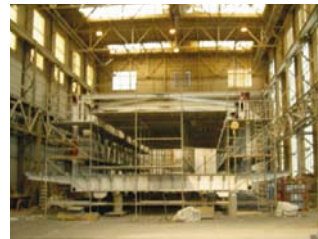
(1) A new bridge is being painted in the workshop before transportation. An enclosure protects the fresh paint from the environment and a dehumidifier regulates the climate.
