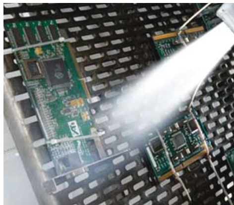
Water damage on pcb's can be cleaned with CO 2 .
