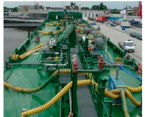
Ventilation and heating of a cargo hold.
