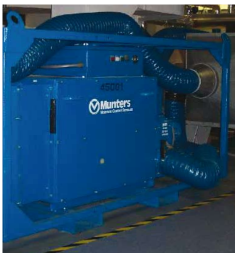
A dehumidifier from Munters helps to reduce moisture in the air.
